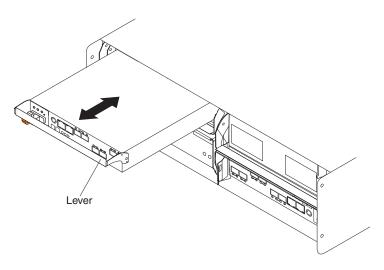
Figure 16. Removing and replacing a controller
